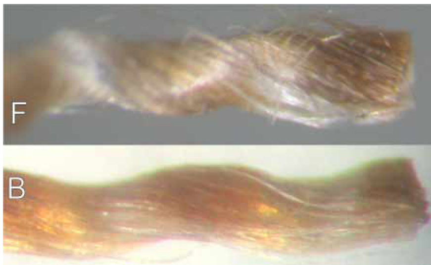
Fig. 8. (Color online) Single yarn of linen F (above) and linen B (below) after irradiation.
